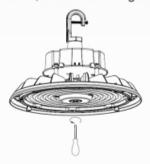
3.Screw the sensor into the base, as shown in Figure 3.
