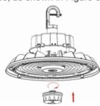
2.Remove the plug screw, as shown in Figure 2.
